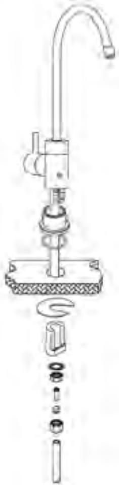
Figure 16: Air Gap Spigot Assembly (Lead Free)\* (treated water spigot)
