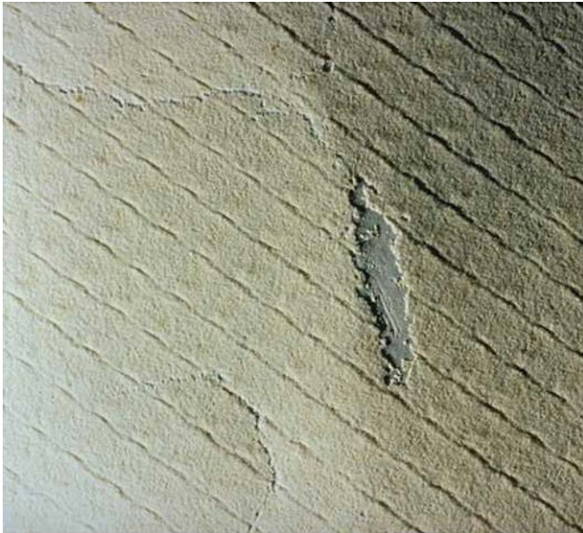
Figure 8.7 Picture of scaled membrane surface with imprints from the feed spacer
