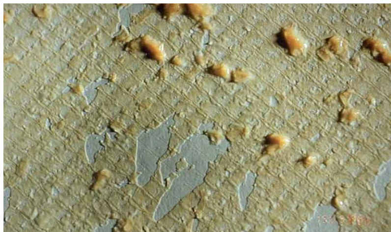
Figure 8.4 Picture of biofilm on membrane surface
