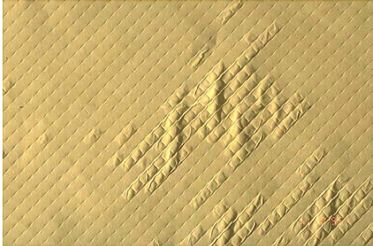
Figure 8.8 Picture of membrane with permeate backpressure damage
