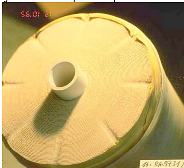
Figure 8.9 The endcap has been pushed off
