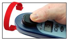
**READ** result displayed on the iDip® and in the app. To save your results and make available for emailing, continue on page 11 of your manual. After testing is complete, rinse CELL immediately.
