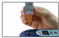
Place the Cell Cover onto the CELL. Press READ and a 20 second countdown begins. Turn the meter upside-down repetitively during the 20 seconds. When the timer displays "1", place the iDip® on a flat surface. The LCD Display will flash "---" and begin counting up for 120 seconds. Make sure your smart device does not go to sleep.
