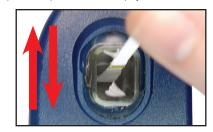
The LCD Display will flash "---" and begin counting up for 20 seconds. During this time, shake the bottle of eXact® Reagent Mn.
