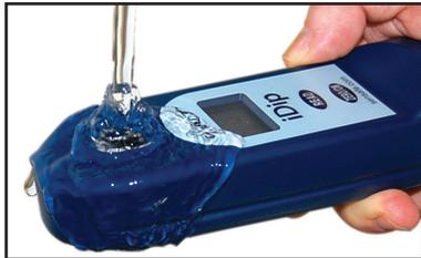
**8** Press **'ZERO/ON'** and the iDip® display reads 0<sub>PPM</sub> indicating the meter is ready to test.
