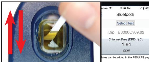
**10** Tap **'SELECT Test'** at the top. Tap Chlorine, Combined (DPD-3) CL. The iDip and app will both display Combined Chlorine.
