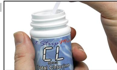
**13** Press **'READ'** to initiate a 20 second countdown and simultaneously **DIP** the test strip by submerging all pads in the sample then use a gentle constant back and forth motion (2 strokes per second) until the timer displays "1". Remove and discard the strip.
