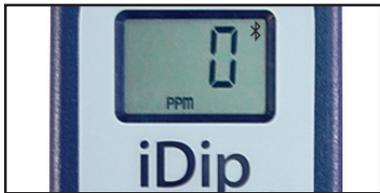
**9** Press **'READ'** to initiate a 20 second countdown and simultaneously **DIP** the test strip by submerging all pads in the sample then use a gentle constant back and forth motion (2 strokes per second) until the timer displays "1". Remove and discard the strip. **READ** result displayed as Free Chlorine. **DO NOT** empty CELL, continue to step 10 to get result as Combined Chlorine.
