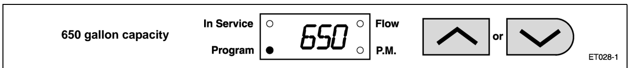
Figure 4: Set Treated Water Capacity
