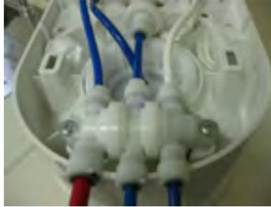
**Figure 13: Input/Output (I/O) Valve**
