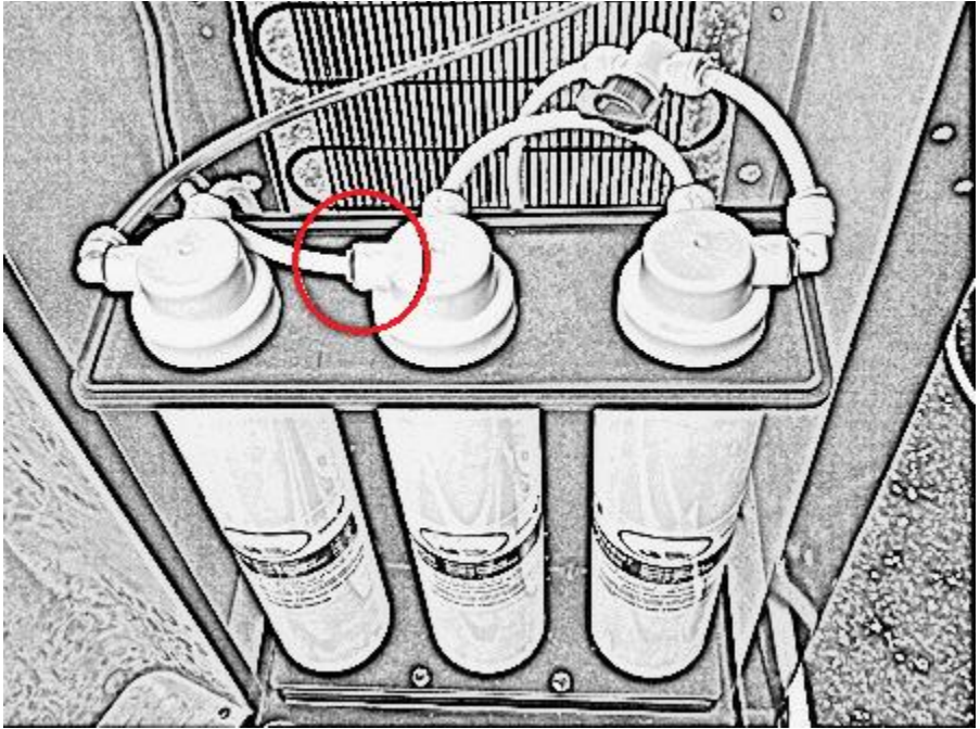
Figure 6 Filter configuration model “F” with cooler door opened
