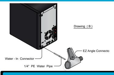
**2-** Connect the 1/4" PE water line between the EZ Angle Connector and the Water In Connector on the back of your H2O-PRO. See drawing (B) .
