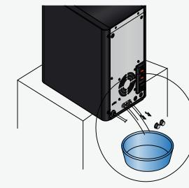
2. Remove the caps on top of the hot water and cold water drains. The remaining water in the tanks will drain out. Cleaning may start when both tanks are emptied. Please put the caps back when cleaning is done.
