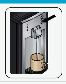
1- After water line is connected, please plug in the water cooler to an electrical outlet. Push any water button to begin filling the water tanks. Please wait at least 5 minutes, before pushing the hot water button, to check that water is dispensing. DO NOT TURN ON HOT WATER POWER SWITCH UNTIL WATER IS DIPENSING FROM HOT WATER BUTTON.
