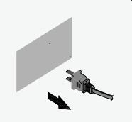
1. Please make sure the machine is completely disconnected from electricity before cleaning.
